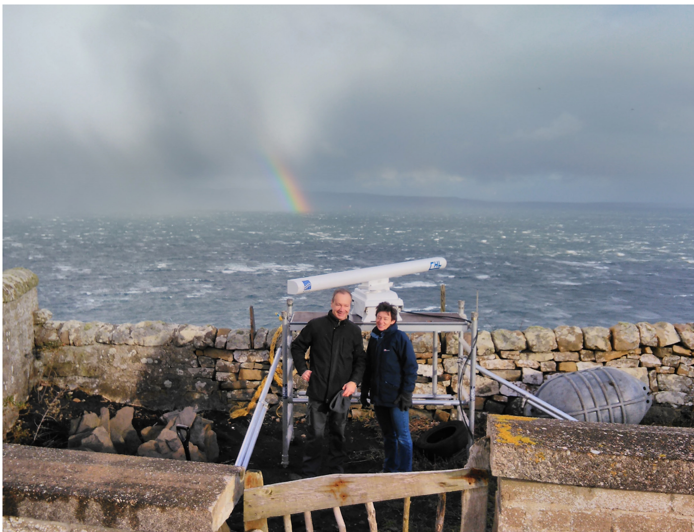
Using X-band radar at Dunnet Head to characterize the sea surface; Dr Philippe Gleizon (l) and Clare MacDowell (r)
