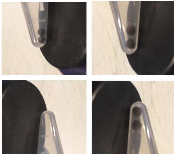
Fig. 5. Two different tubes (left and right) containing gunshot pellets, with the tube tip held against a fridge magnet with the tip oriented downwards (top) and then inverted so that the tip points upwards (bottom). The tube on the left contains non-magnetic shot and that on the right contains magnetic shot.
