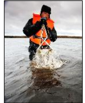
Using the sediment grab to look at invertebrates in lochs on the Forsinard reserve
