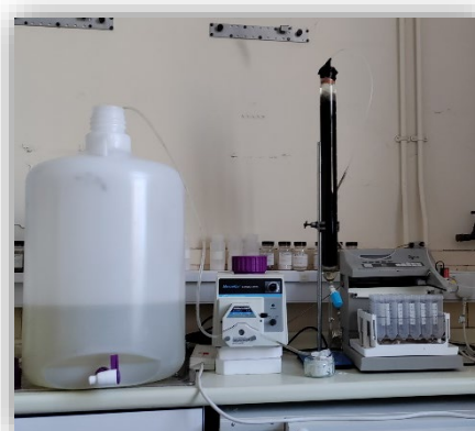
LAB-SCALE FILTRATION SYSTEM
